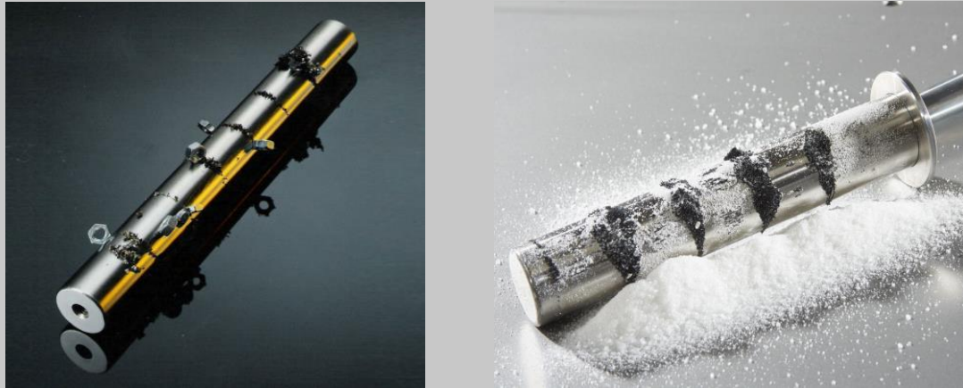
Magnetic bars used in magnetic separation systems. Particles captured collect on the rod near the pole plates because the Force Index is highest there.
