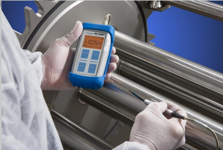
A flux density meter (upper left) and its application to a magnetic separation system (bottom right)
