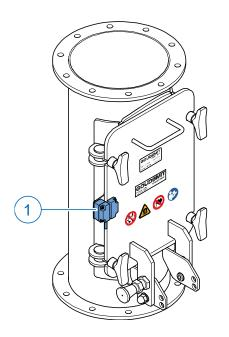
By default, the device is equipped with a door sensor [1] that detects when the door is in the open or closed position.
