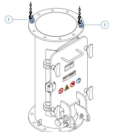
Lift the device out of the crate evenly. Use a hoisting unit that supports the device.
